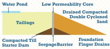
The underlying dam foundation conditions will be examined and designed to safely accommodate the expected load of these structures
