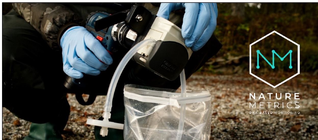
Photo 2.2-3: Field-Filter Method (Vampire Sampler) Setup Used at all Sites Sampled in 2023. Note: The majority of 2023 samples were taken directly from the watercourse and the sample bag was only used when turbidity was high. Photo obtained from the Nature Metrics Vampire Sampler document (Nature Metrics 2023).
